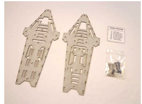
Remove the items from the "Main Frame" Bag. Initially the two large frame pieces (Top and Bottom Deck) and the 18 button head screws is what will be needed
