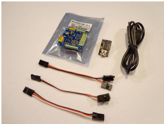
This build will use the MultiWii SE v2.5 Flight Control (FC) Board, available from Twisted Hobbys, comes with the accessories shown
