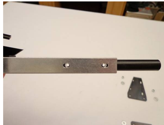
It does not have to slide freely, but should go in and out with only a slight amount of pressure. Line the holes up with the slots. Slots are used in a later step to adjust the end play in the Tail Box
