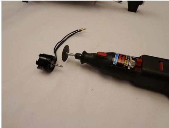
Prepare the Tail Motor for mounting. The Shaft must be shortened
