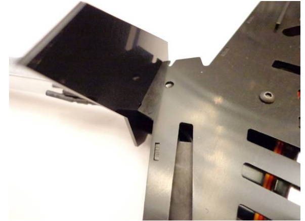
Pivot the Boom slightly forward so that the Leg can engage the front set of slots
