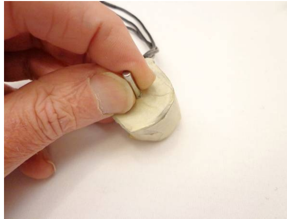
Wrap the motor with tape to completely seal it off so that no shavings get inside during the shaft cutting process
