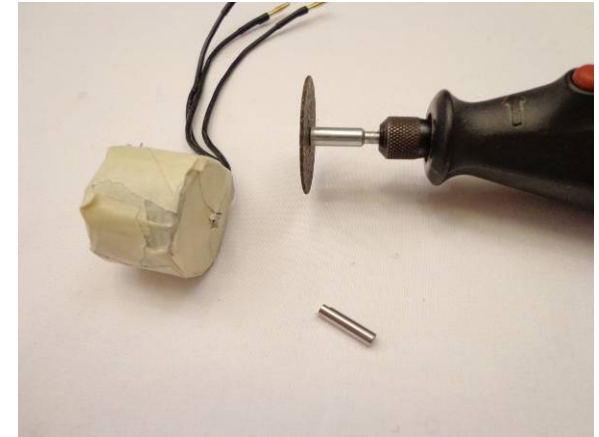
Cut the Shaft..... leave about 3/16" to 1/4" from the base of the motor
