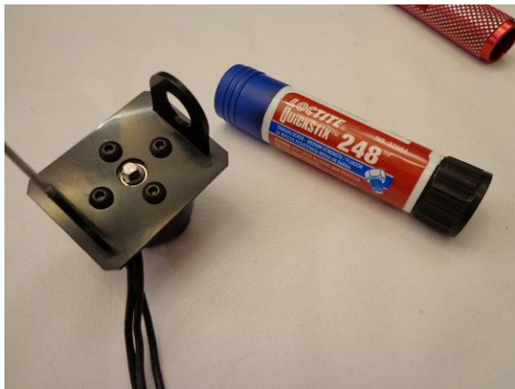
Secure the motor to the Motor Plate. Use thread locker and make sure the motor spins freely.
