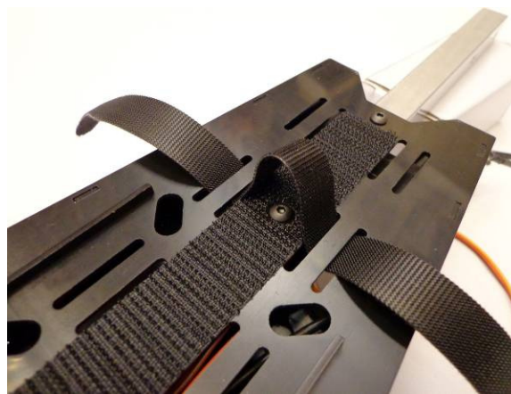
Install the screws to secure the Bottom Deck. Loosely again, starting from the nose and working back. Enlarge any holes as necessary for alignment
