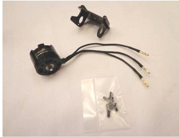
Find the bag of hardware that contains the five screws that were included in the Tail Bag. The four button head screws will be used to attach the motor to the Motor Plate
