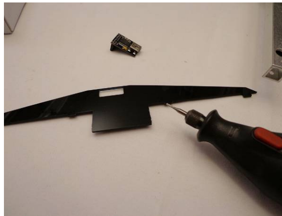
Hole added with a motor tool for the USB adapter. Note - this slot was added in later releases of the model
