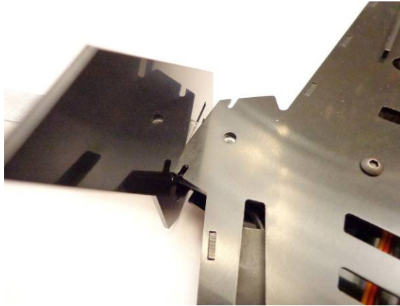
Line up the slots in the Leg with the material thickness of the Top and Bottom Decks
