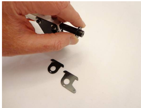
Check the fit of the Spacer to the Tail Pivot Shaft as shown. It should slide freely, a little friction is okay
