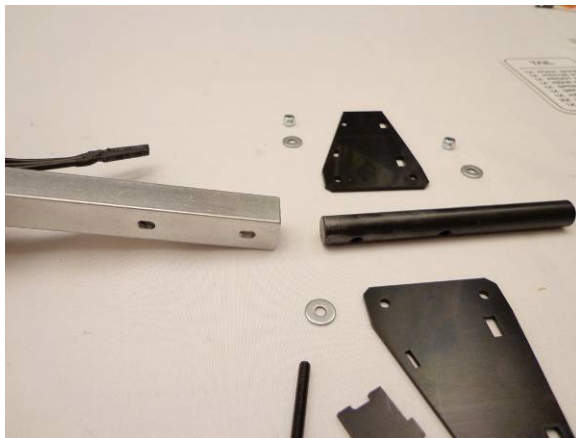
Slide the Pivot Shaft into the opening in the back of the Rear Boom. Note - End with the holes goes in first
